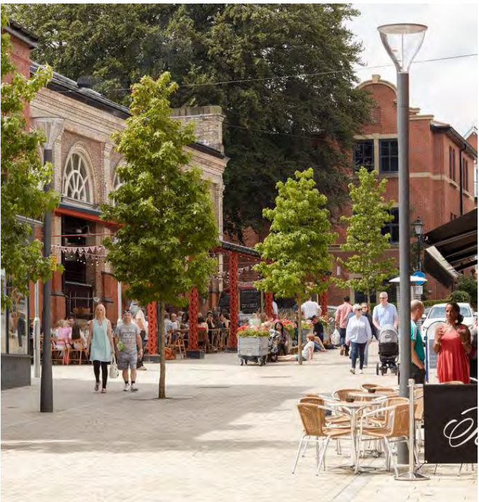
Image 4.9: Areas of high pedestrian activity in town centre include lower level lighting columns (Altrincham, Manchester).
