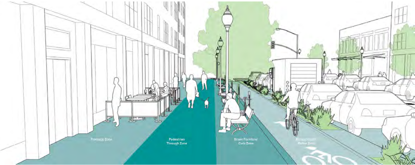
Image 2.1: Diagram outlining the key zones that organise the pavement and establish a clear and legible pedestrian framework.
